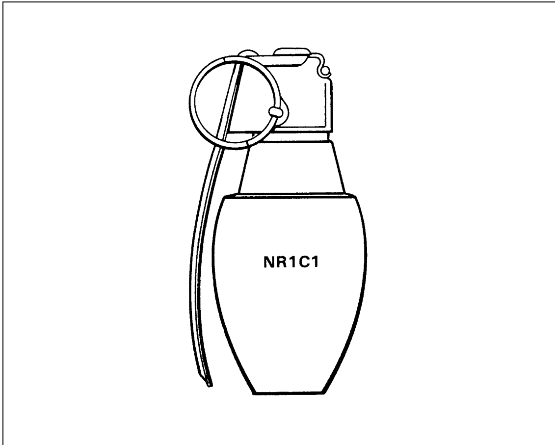
Figure F-4. NR1C1 fragmentation hand grenade.
